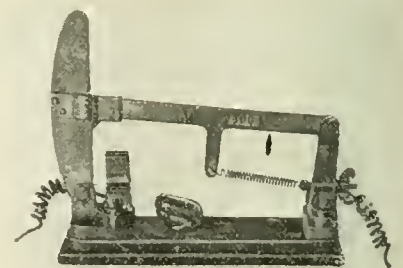
FIG. C. THE CIRCUIT BREAKER IN THE TRACK CIRCUIT.
